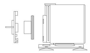
5. Clasp the impeller blades with needle nose pliers and slowly pull the impeller from the impeller chamber.
